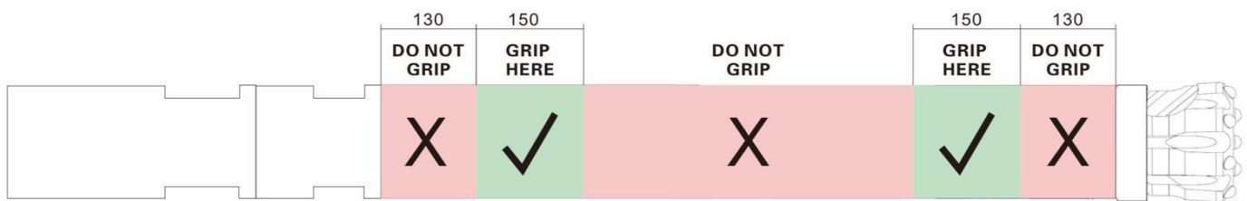
Figure 1: Gripping Locations for BD DRILL Reverse Circulation Hammer Lubrication
