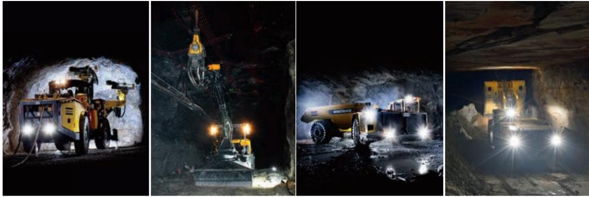
The same fleet of equipment can be used for both development of the cut and fill mine and for production.
