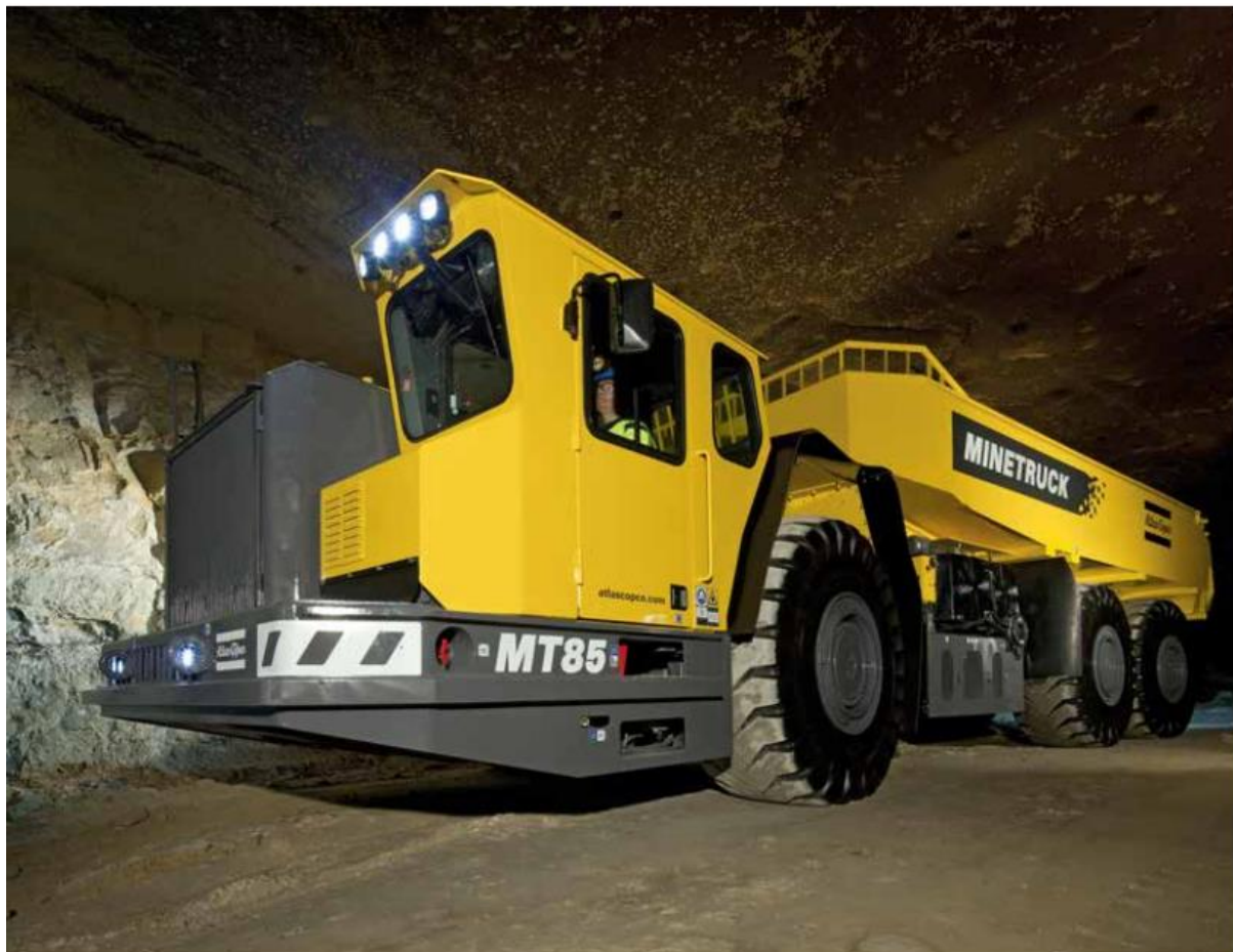
Modern mine vehicles are capable of severe road grades, although a maximum of 12% is recommended to avoid high maintenance costs. Well maintained roads can also significantly reduce the cost of tire replacements.
