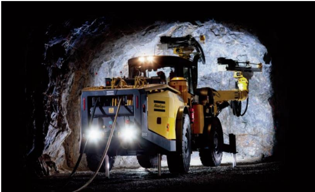
Precision drilling, maximized uptime and several levels of automation are some of the key features of Atlas Copco's range of Boomer drill rigs.
