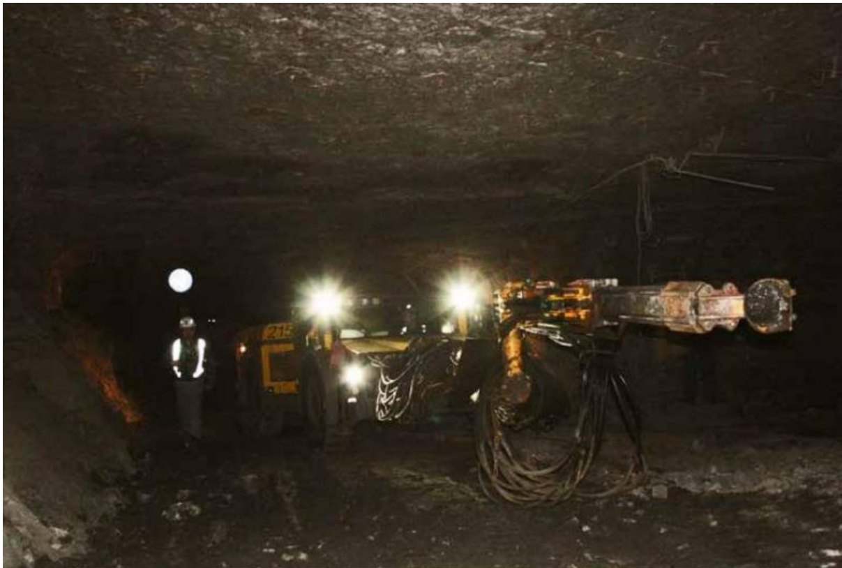
Low profile drifts are expected to become more common as existing mines increase their operational depths.
